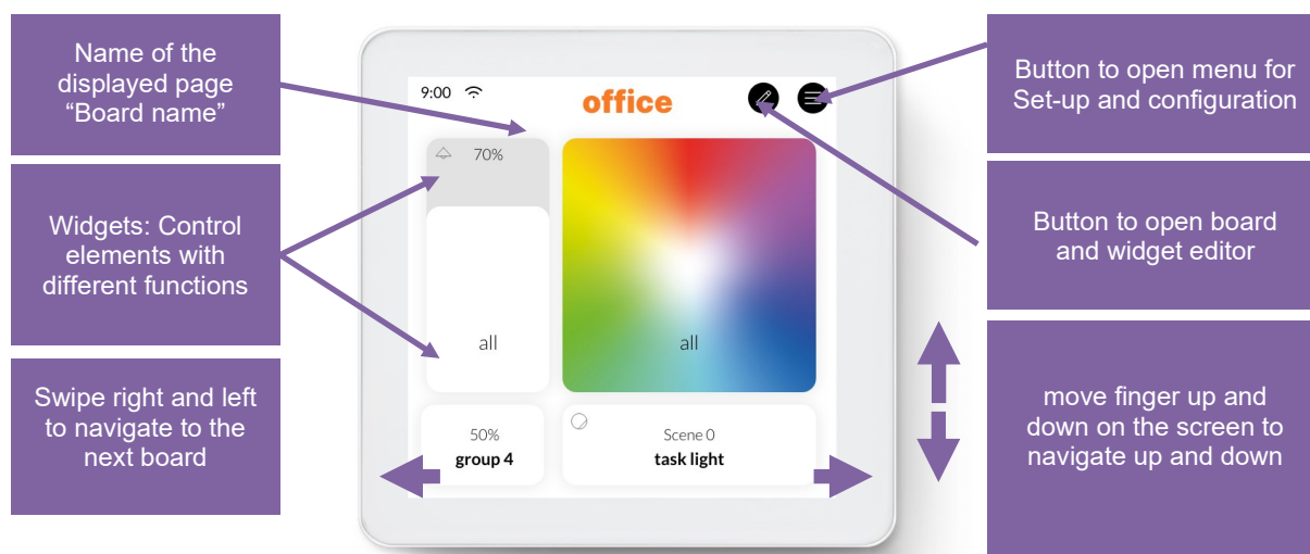
Figure 4 User Interface for Light Control DALI Display 4"
